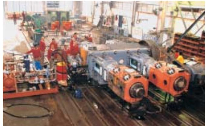
*4HF/3 Compressor for IOC Panipat Refinery supplied by BPCL*
