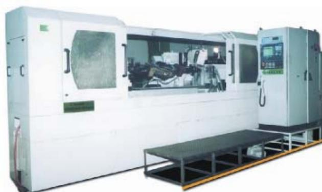
CNC Axle grinding machine manufactured by HMT
