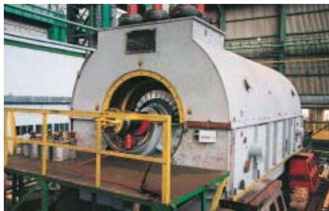
*Turbo Generator for Libya Project (4x150 MW) manufactured by BHEL.*
