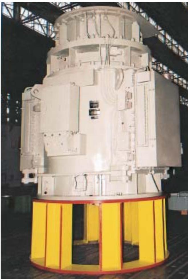
*Largest capacity (6MW, 1500 RPM, 6.6KV) Vertical motor produced by BHEL.*
