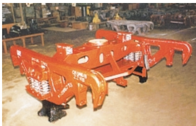
Cast Steel High Speed bogie manufactured by Burn Standard & Co. Ltd.
