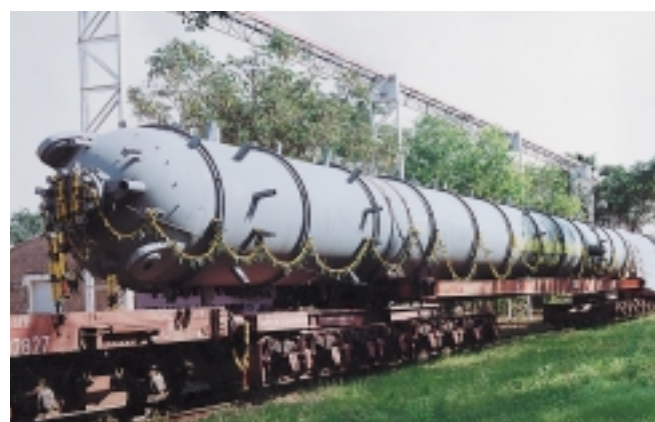
225 M.T. Urea Reactor manufactured by BHPV.
