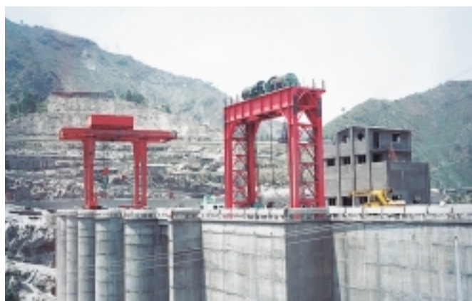
Gantry crane and bulk head emergency host for Chamera project by TSPL
