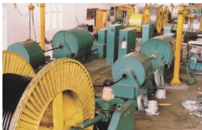
Armouring of Jelly filled cables at Hyderabad Plant of HCL
