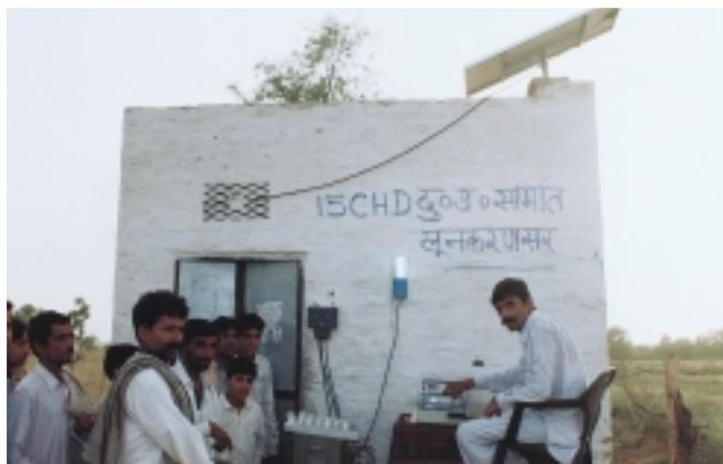
*Solar operated Electronic Milk Testing equipment by REIL.*
