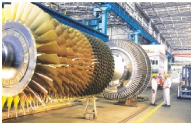
*Gas Turbine rotor on assembly bed at BHEL, Hyderabad.*
