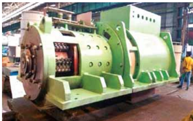
500kW Main Motor Generator (MMG) (assembly of AC & DC machine) for defence application designed & manufactured by BHEL
