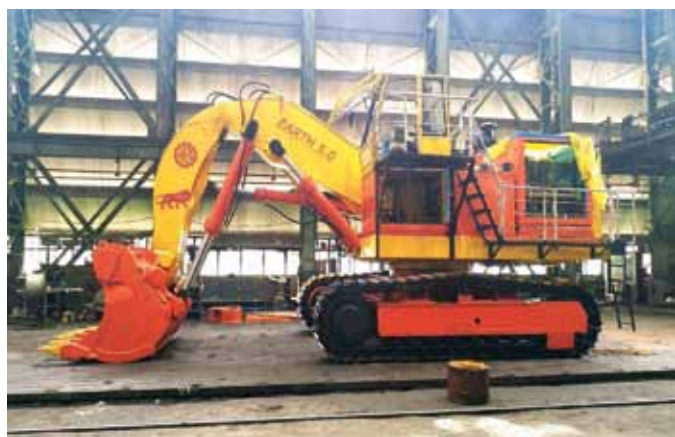
5 Cubic Meter Hydraulic Excavator - HEX 400 developed by Centre of Excellence at HEC Ranchi
