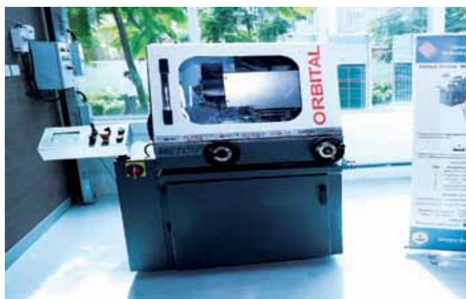
Orbital Motion Abrasive Cutting Machine developed by Centre of Excellence at IIT, Madras
