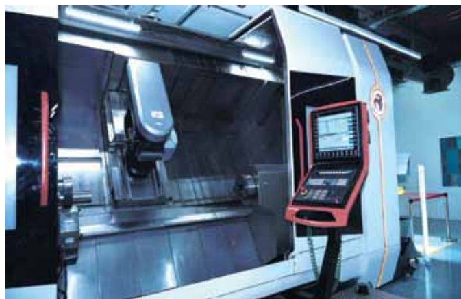
5-axis Multi Tasking machine developed by Centre of Excellence at IIT, Madras
