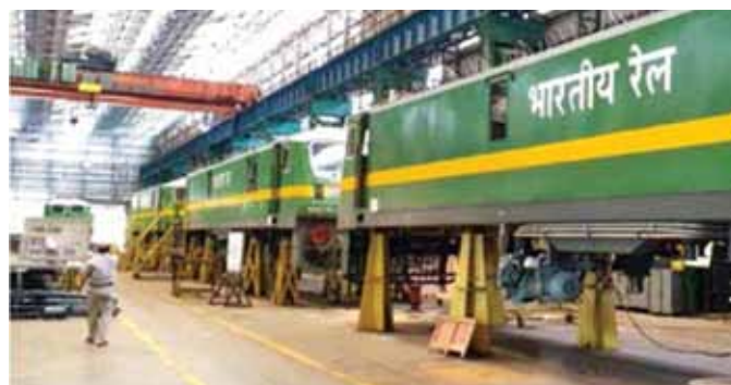
WAG9 locomotives under manufacture for Indian Railways at TP Jhansi
