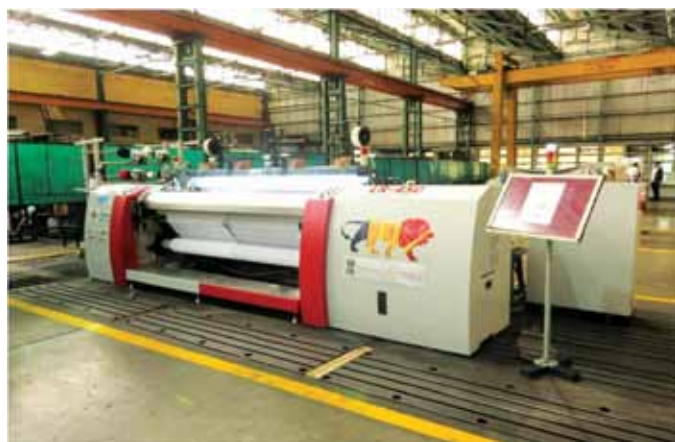
Shuttle less rapier loom of 450 RPM developed by Centre of Excellence at CMTI, Bengaluru
