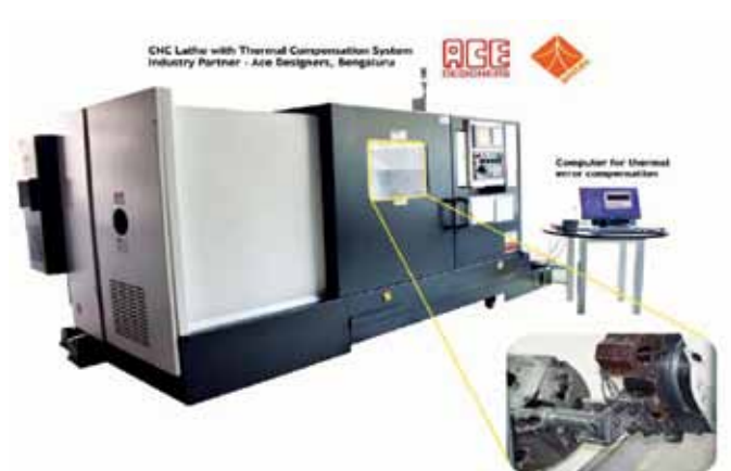
Thermal Compensation System for CNC Turning Centre developed by Centre of Excellence at IIT, Madras
