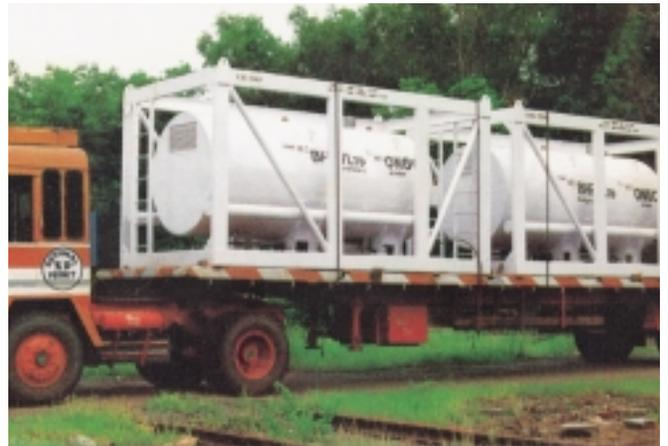
*Super Insulated Skid mounted Cryogenic Tanks by BHPV.*
